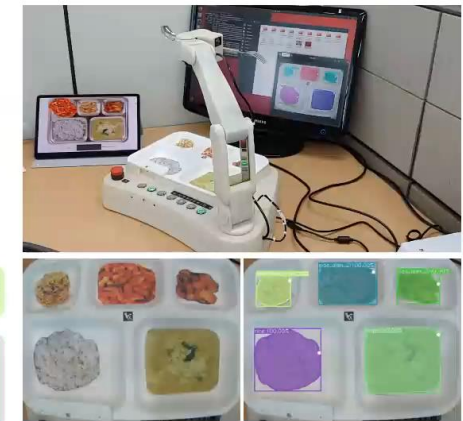
Fig 2. (a) original image. (b) segmentation result
