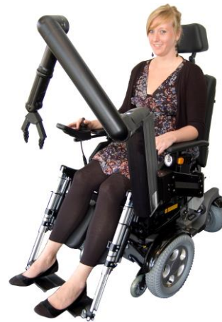
MANUS ARM, iARM: A successful "commercial" robotic arm. (Exact Dynamics, NL, 1990)
